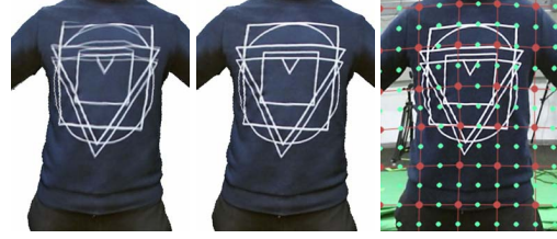
Figure 6. Left: optimization only at the finest scale. Middle: our multi-grid approach. The thin line patterns are aligned. Right: an illustration of the control points from a coarser scale (red dots) and the next finer scale (green dots).
