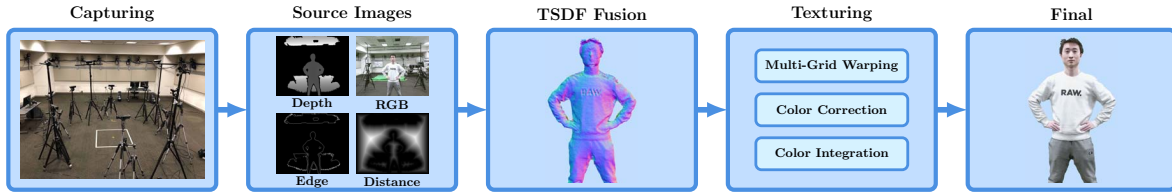
Figure 1. Overview of our geometry and texture reconstruction pipeline.
