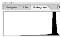
This image has a lot of highlight information and is lacking in shadow detail
