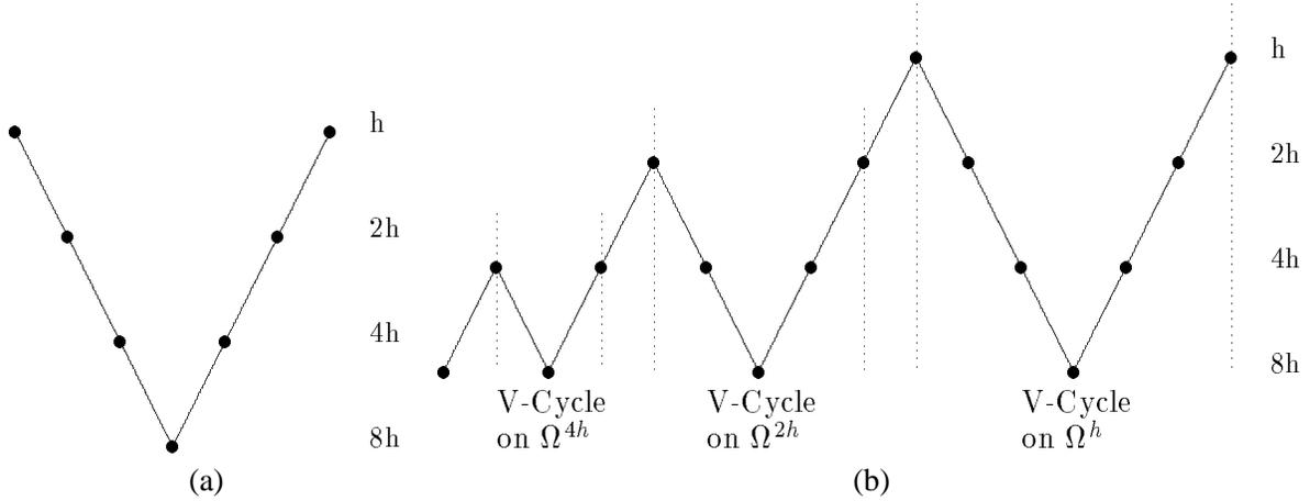
Figure 4: Relaxation schedules for (a) V-Cycle (b) Full Multigrid V-Cycle, all on four levels
