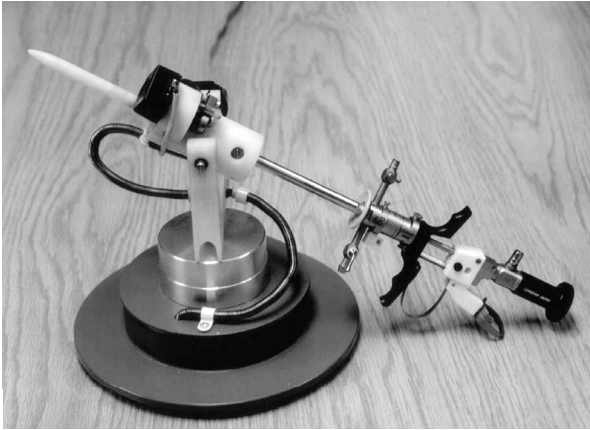
FIG. 3. Hardware interface device for lower urinary tract endoscopy simulation, which allows four degrees of freedom and provides haptic experience to simulate tissue resistance.
