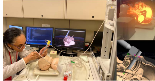
Figure 1: The overview of our XR system setup in the data collection study (left). The top right figure shows a registered sagittal cross-section of the CT-scanned manikin in the Hololens; the bottom right figure shows the instant feedback with performance parameters.
