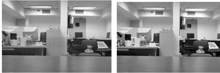
Fig. 1. Left: Background estimation with averaging, Right: Refined with large and small threshold
