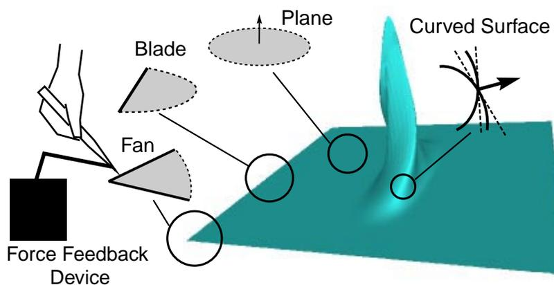
**Fig. 1 Feature-Based Haptic Rendering**
