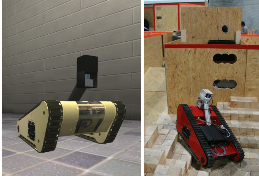
Figure 5.1: Skid-Steered Vehicle . A skid-steered vehicles refer to a tracked or wheeled ground vehicle that is maneuvered using differential control of the left and right tracks or wheels. The picture on the left shows the simulated skid-steered vehicle used for this research that was modeled in USARSim. The picture on the right shows the actual vehicle.
