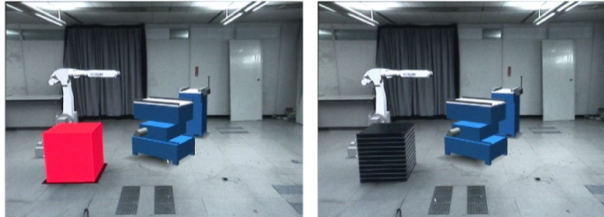
(b) Using mask objects (a real box with a virtual robot) [Lee et al., 2008a]
