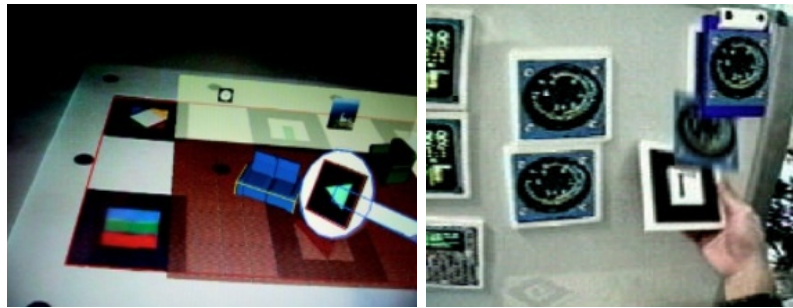
Figure 7.5: Examples of time multiplexed (left: VOMAR [Kato et al., 2000]) and space multiplexed (right: Tiles [Poupyrev et al., 2002]) Tangible AR interfaces.
