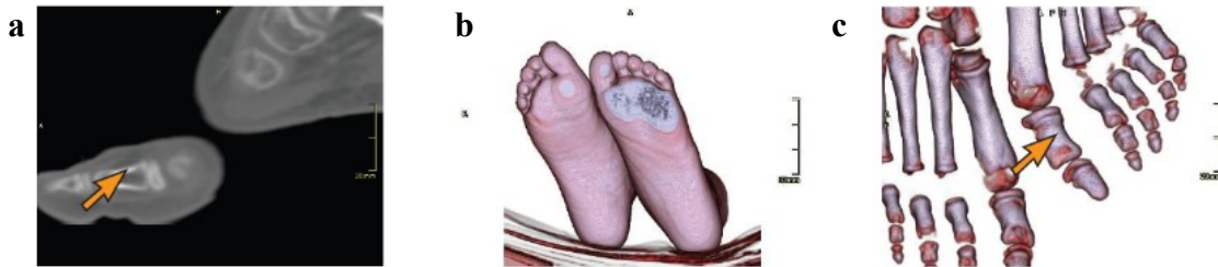
Figure 2-3: 2D slice picking. 2D slice picking (a) results in the optimal transfer function and viewing direction for the dataset (b). The same picked point is made visible and pointed at in the optimal 3D rendering (c). [26]
